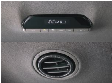
Rear Ventilation System
